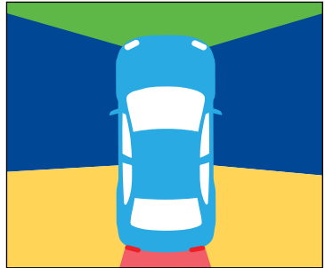
Know the areas of your vehicle. Green is What Is Ahead. Blue is What Is At Your Side. Yellow is Blind Spots/No Zones. Red is What Is Behind You.
